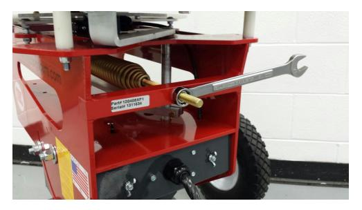
**Step 15** – The pull cord or optional radio release can now be connected to the machine. The manual pull cord or optional wireless release is connected to the yellow-ended cord plug.
